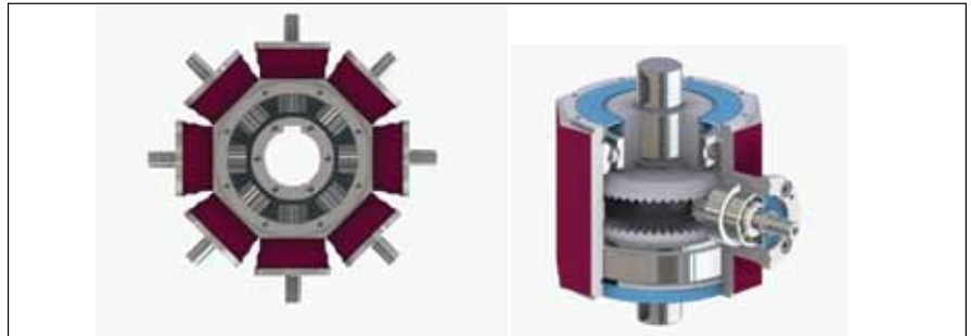
Figure 12—Up to eight pinion shafts on one layer can be mounted (left). Depending on the application, only one output may be needed. If required, it can be combined with a second face gear.
