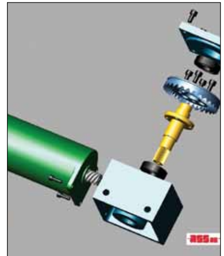
Figure 5—Automatic door moving system with Cylkro transmission.
